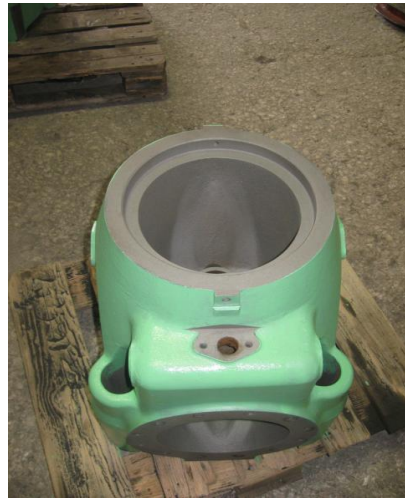
Picture Exhaust Valve Housing of 50MC
