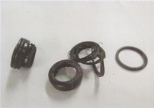
Damaged synthetic piston (POM: Polyacetal)
