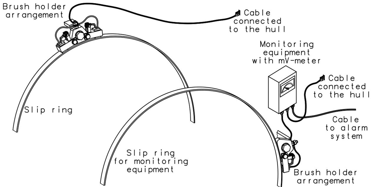
The slip rings should be made of solid silver or back-up rings of copper with a silver layer all over. The expected life span of the silver layer on the slip rings should be minimum 5 years.
