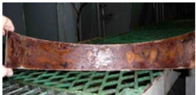
*Heavy corrosion on the back side of the slip ring*
