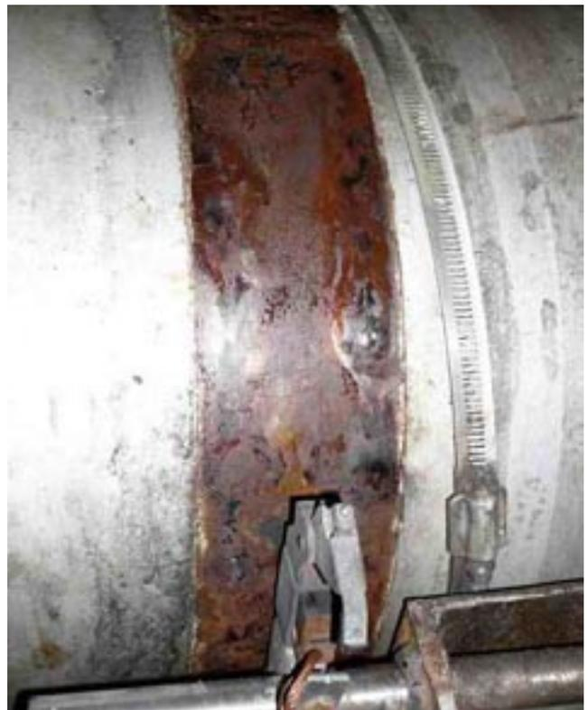
*Corrosion hiding behind the slip ring*
