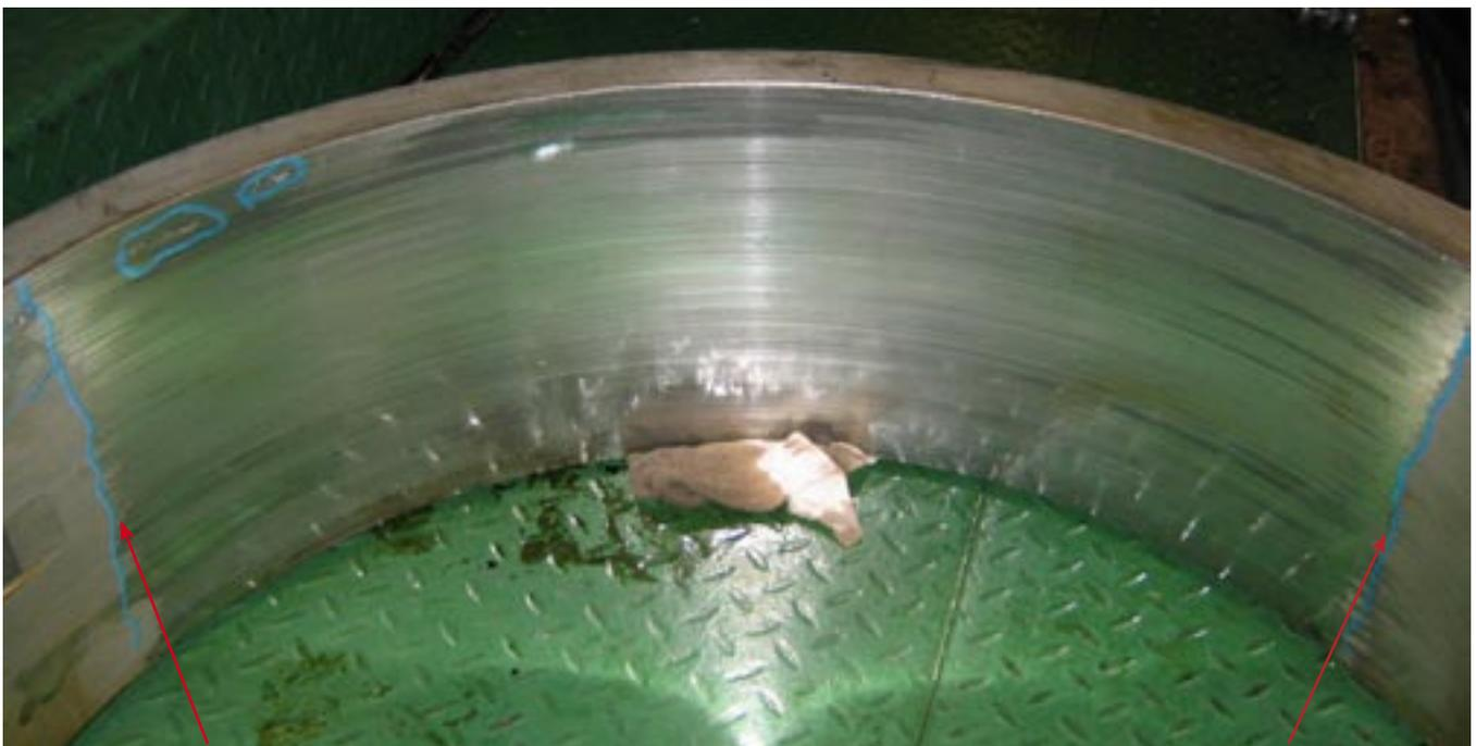
*Corresponding main bearing lower shell with wide spread journal imprint. 0.5 mm of the shell is worn off between the two distinct, visible lines.*
